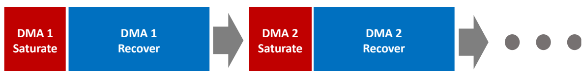
Figure 11-Progressive transitioning of district metered areas (DMAs) ensures the availability of water and human resources during the transition stage.
